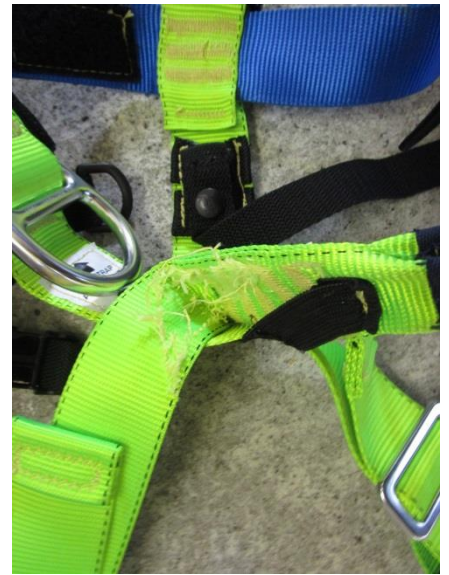
ST2018-5 PRSH1196-FR FRONT NECK 10KN STATIC LOAD SPV Data(kg) 23/01/2018 2:49:32 p.m. Final Value 0
